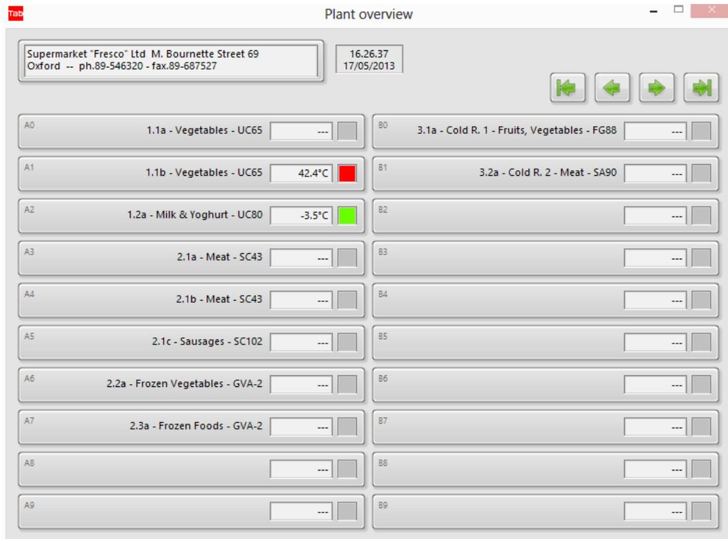
The units appear arranged in 26 columns (A...Z) of 10 elements (0...9). In order to get the visible columns scroll, press the buttons with the arrows, at the top right page.
